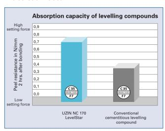
The absorbency of the new premium levelling compound is approx. twice as high as previous levelling compounds. The open time of the adhesive during the laying is considerably reduced in comparison with usual compounds. The installer of the covering works far faster and the overall appearance of the finished floor covering surface is very smooth and flat.
